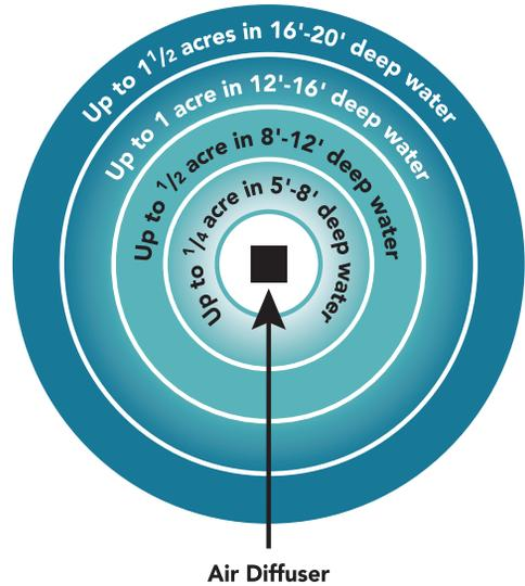
*The deeper an air diffuser is located, the more "boiling action" it will create and a larger area will be aerated.*
